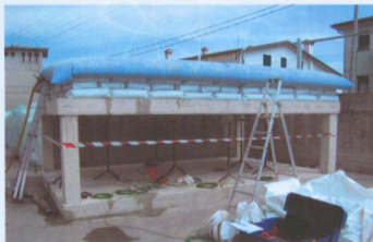
Photo of floor load arrangement (maximum load of 550 kg/m 2 )
